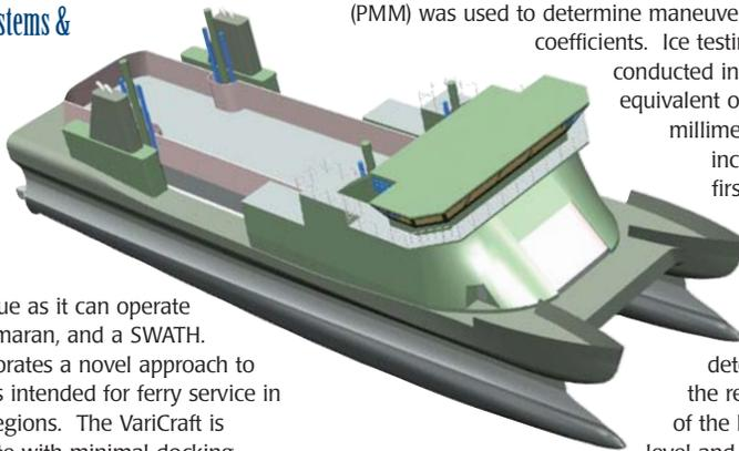
of the hull, open water tests determined the hull resistance of the hull propulsion characteristics in calm water. Oceanic's Planer Motion Mechanism (PMM) was used to determine maneuvering coefficients. Ice testing was
