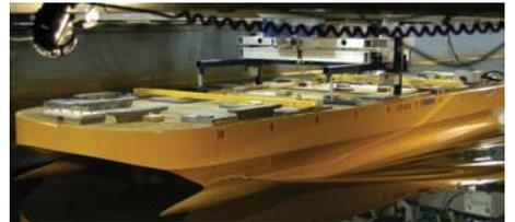
resistance, ice resistance, speed loss in waves, and seakeeping while motions and hull loads were being measured.
