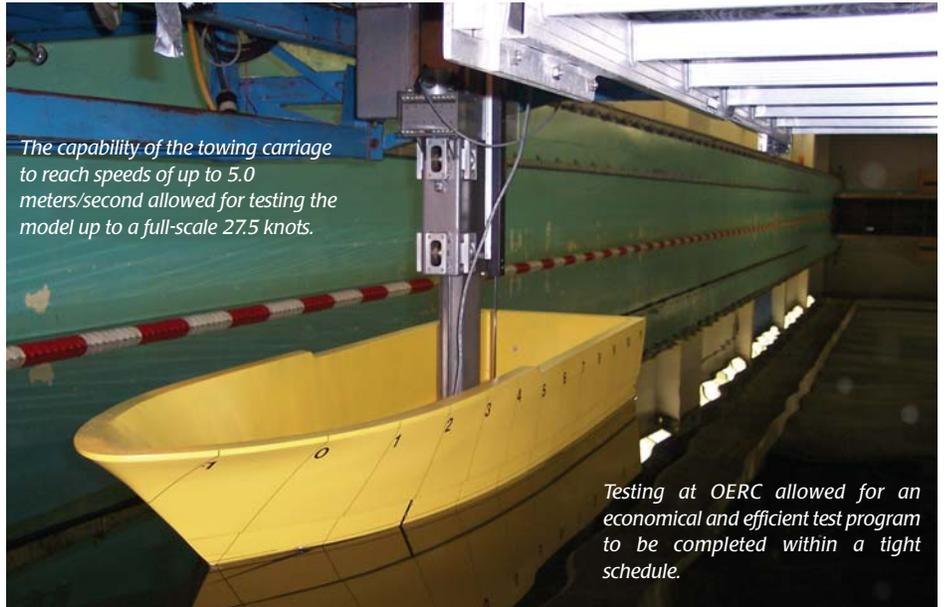
The capability of the towing carriage to reach speeds of up to 5.0 meters/second allowed for testing the model up to a full-scale 27.5 knots.
